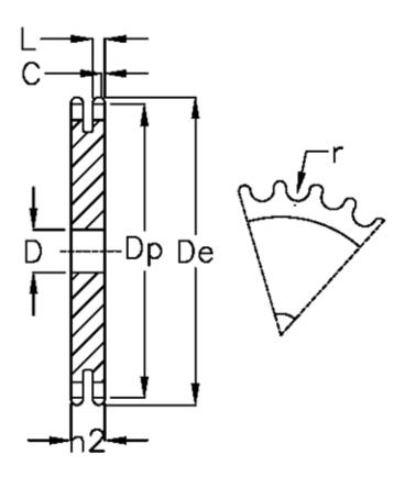
C = 4 D = 25 De = 248.3 Dp = 233.17 For chain size = 1 1/4 x 3/4 For chain type = 20 B-2 h2 = 54.6
